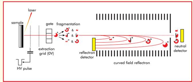
Figure 1: Schematic of the curved field reflectron
