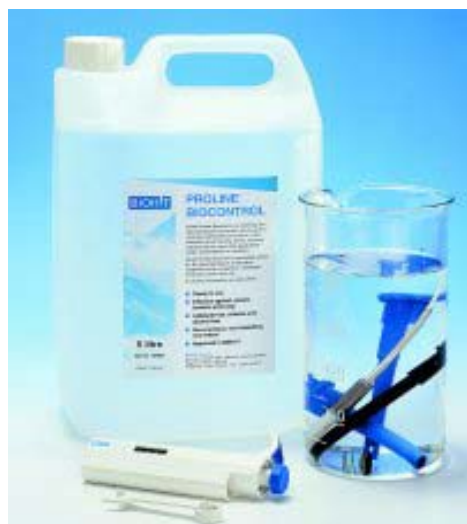
Fig. 4. Decontamination is done easily by spraying with specific decontamination solutions, such as the Biohit Proline Biocontrol. For complete decontamination, the tip cone parts can be soaked in the solution for 30 minutes.
