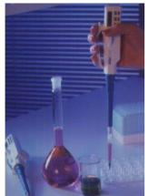
Figure 1. Automatic dilution of samples in pipettor tip using Biohit Proline Electronic pipettor saves time and replaces the double operation of a mechanical pipettor.
