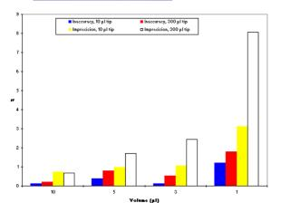
Figure 2. Comparison of inaccuracy and imprecision using 10 and 300  $\mu$ l tip in dispensing 1, 3, 5 and 10  $\mu$ l.
