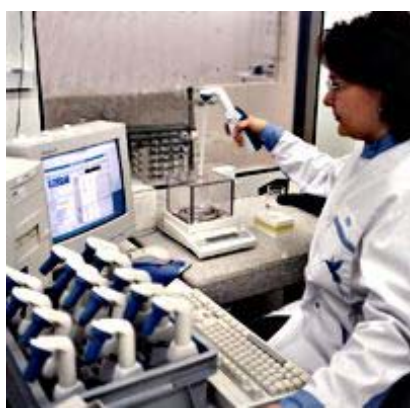
Fig. 1. Performance checking of a pipettor using the gravimetric method monitored by a computer.
